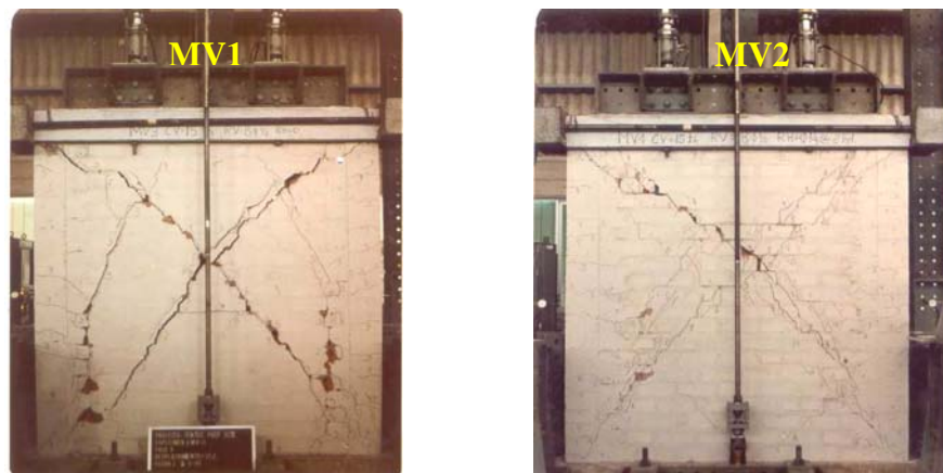
Figure 5. Confined walls tested under cyclic load and constant axial load; left: wall MV1 without horizontal reinforcement, and right: wall MV2 with horizontal reinforcement.
