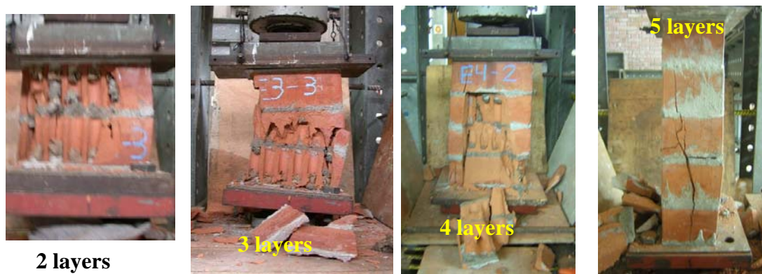
Figure 9. Tested prisms of industrial clay units (IC).
