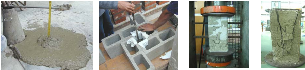
Figure 5. Grout preparation and tests, from left to right: slump measure, casting with filtering paper, test machine and typical failure of a grout specimen.
