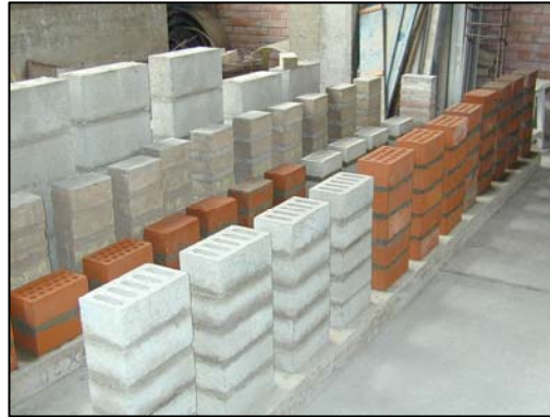
Figure 6. Masonry prisms built of clay bricks (AC and IC), concrete bricks (ICo), and concrete blocks (BIC).
