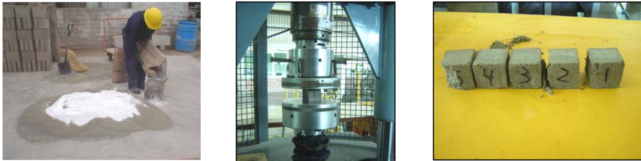
Figure 4. Mortar preparation and cube tests, left to right: mixture of cement, lime and sand, test of the small cubes in compression, and some of the cubes already tested.
