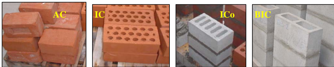
Figure 2. Masonry units used in the experimental tests, left to right: 1) AC (artisan clay); 2) IC (industrial clay); 3) ICo (Industrial concrete); 4) BIC (block industrial concrete).
