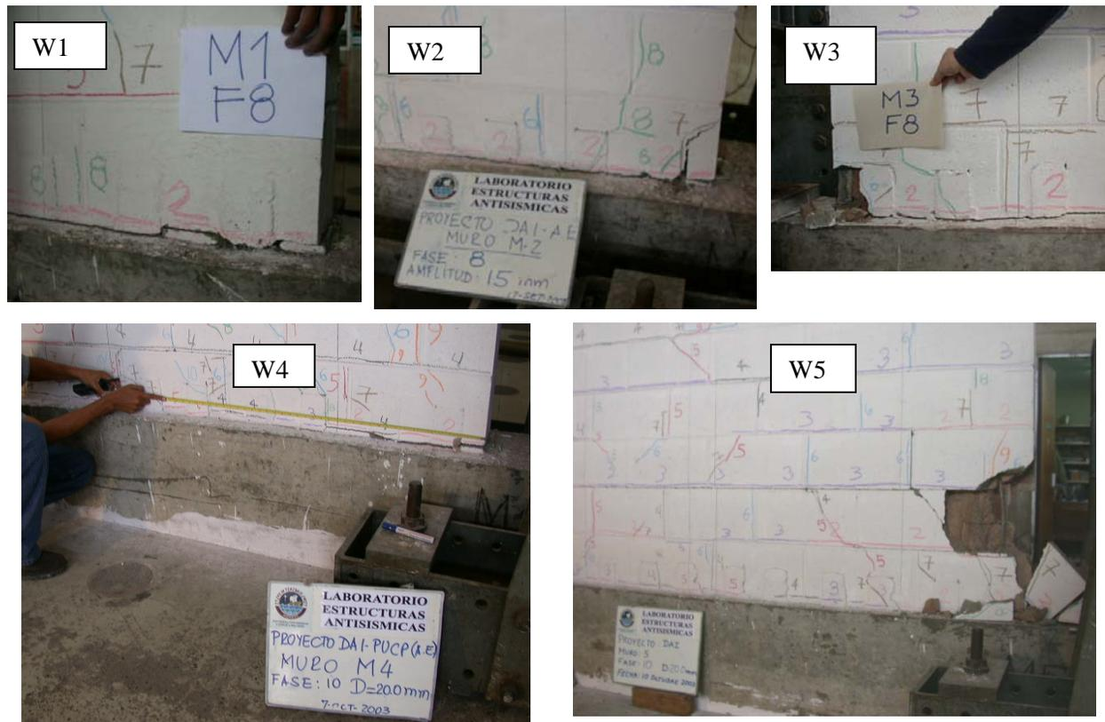
**Figure 12: Walls showing sliding failure at different steps of the test, except W4.**
