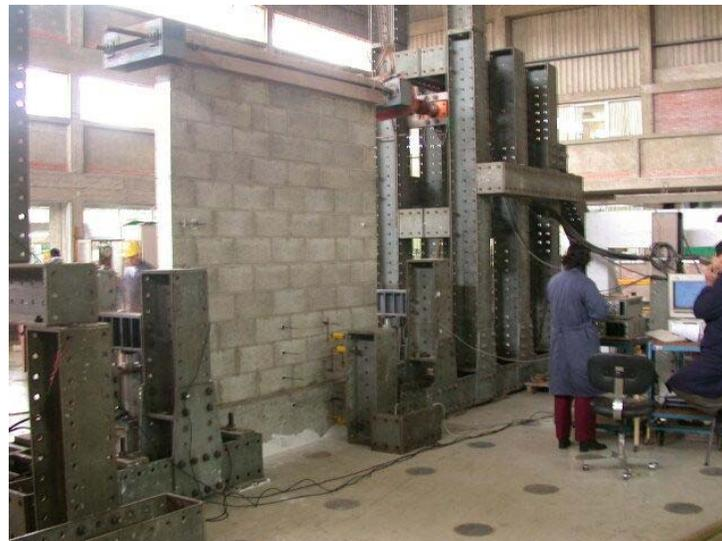
**Figure 10: Test setup for cyclic lateral load**
