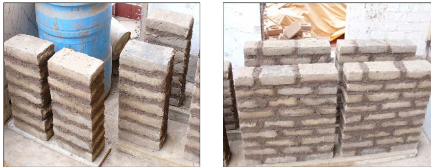
Figure 3: Adobe prisms and small walls
