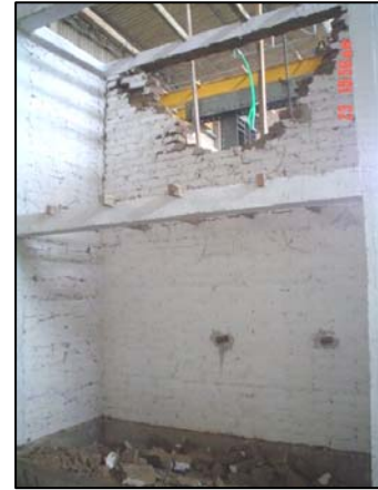
Figure 10: Specimen during step 4 (left) and after step 4 (center and right).
